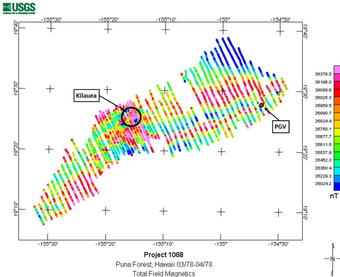
**Figure 3: Map of the 1978 USGS ‘Puna Forest’ airborne magnetic survey with flight lines overlain with Total Field Magnetics.**
