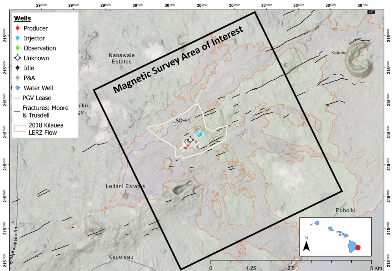
**Figure 4:** Survey AOI from the 2024 Ormat UAS magnetic study, flight lines spaced 100 m, with tie-lines every 400 m.
